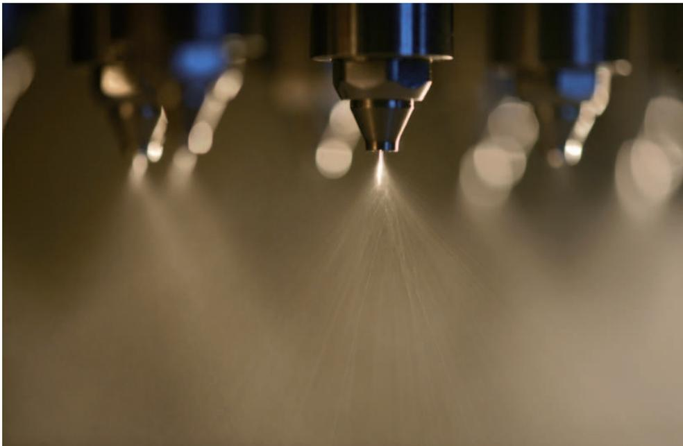
Using the TEKAWE spraying device "TEKA exacto Spray" mainly thinny and liquid substances such as water, release agents and oil can be sprayed exactly and precisely timed.
