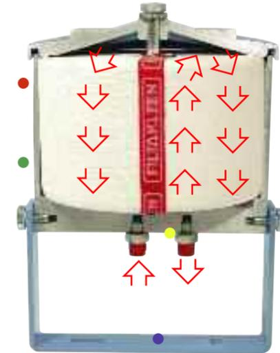
The high tech cartridge gives continuous all round protection against water and ultra-fine debris with contaminated oil entering the filtakleen unit at the base flowing up the centre tube through the 1 micron filter before flowing back to the hydraulic circuit. Flow rates through filter 4.1 l/min to 6.1 l/min depending on unit fitted.
